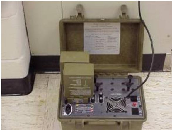
If you get a red fault light when charging the BB-390, with a known good charger, most likely these batteries have been drained and left on the shelf for a few years. We can bring most of them back to life. A little less overall capacity, but they should provide reasonable power for you. Voltages at pins 1-4 and 2-5 are most likely well below 6 volts. So try the following:
